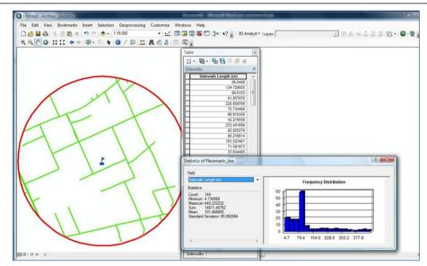
Figure 4 Computer screen shot of the road network layer with sidewalk coverage for a 1 km radius circular buffer testing site obtained within ArcGIS and the summary table with the sidewalk length details (right side).
